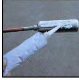
11. Smear silicon grease on the surface of heat pipe condenser. (Used to increase energy transfer efficiency)
