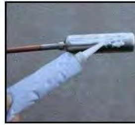
15. Smear silicon grease on the surface of heat pipe condenser. (Used to increase energy transfer efficiency)
