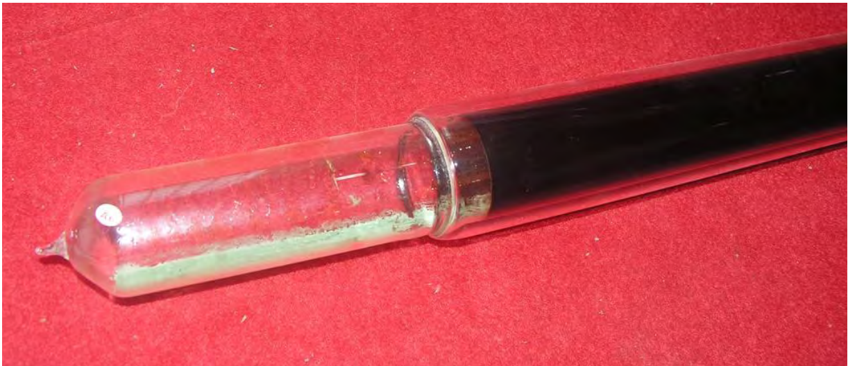
Figure 17: All glass heat pipe condenser end
